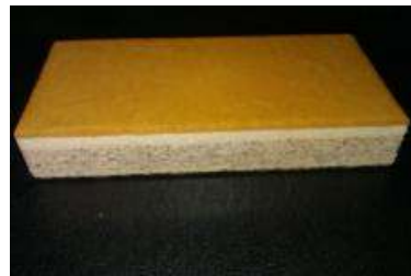
Fig. 2 Composite consist of sand material and resins
