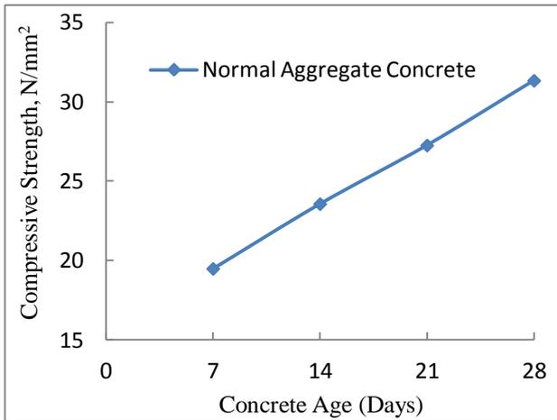
Fig. 1 Compressive strength for normal aggregate concrete (NAC) with 100% ordinary Portland cement.
