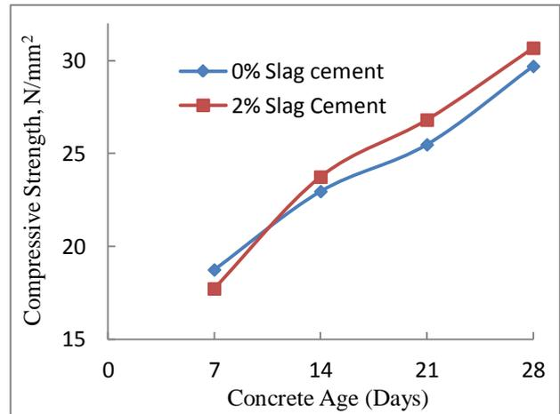
Fig 2 Compressive strength for slag aggregate concrete (SAC) with 2% slag cementitious replacement.
