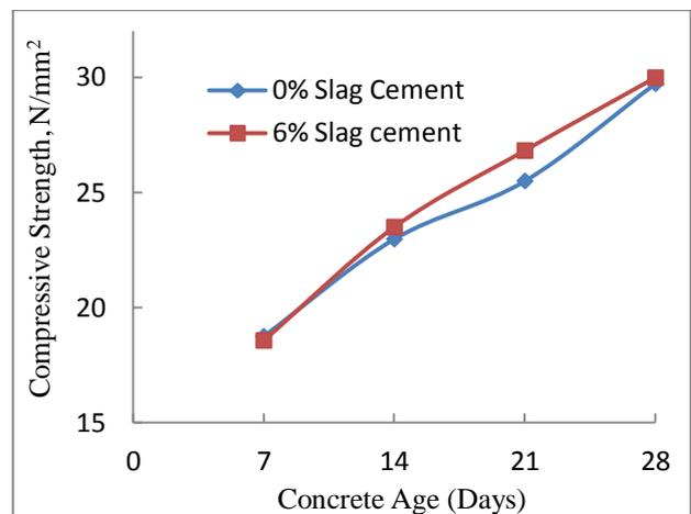
Fig. 4 Compressive Strength for slag aggregate concrete (SAC) with 6% slag cementitious replacement.
