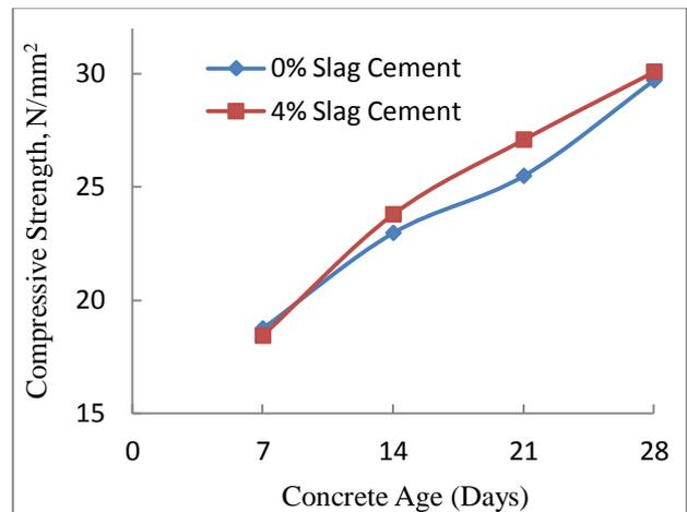
Fig. 3 Compressive strength for slag aggregate concrete (SAC) with 4% slag cementitious replacement.
