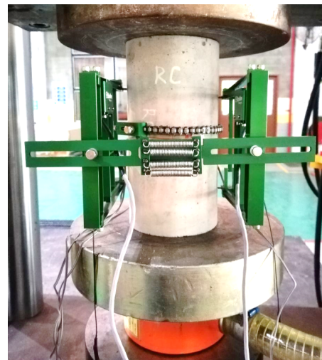
Fig. 2 – Elastic modulus measurement setup
