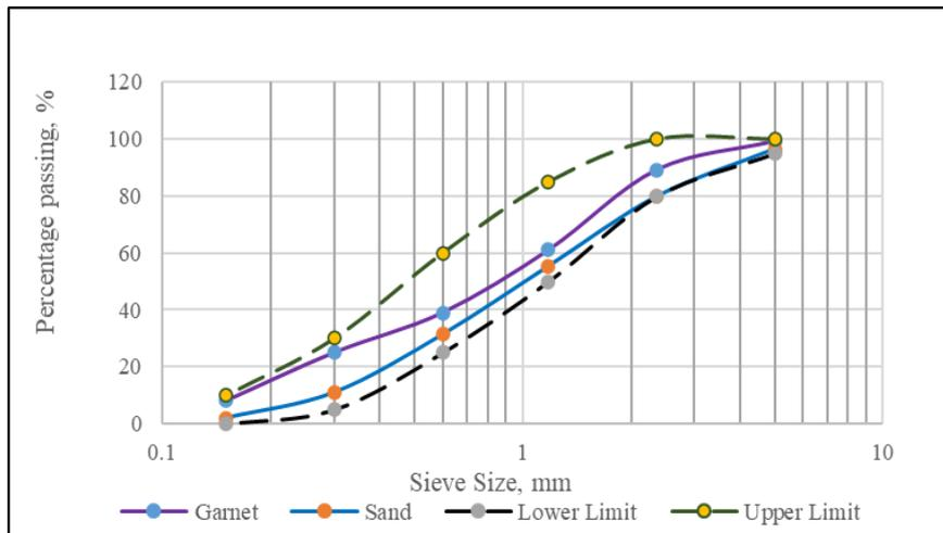
Fig. 2 - Grading curve of fine aggregates and spent garnet
