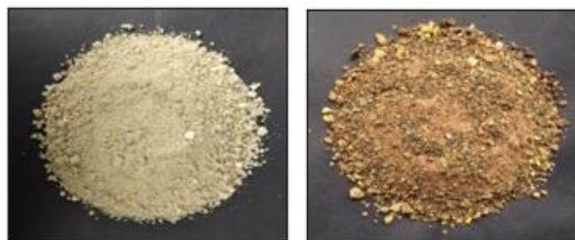
**Fig. 1 - Fine aggregates used (a) River sand and (b) spent garnet**
