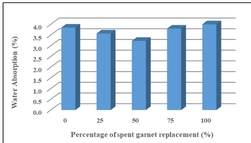
Fig. 7 - Water absorption at 28 days' tests
