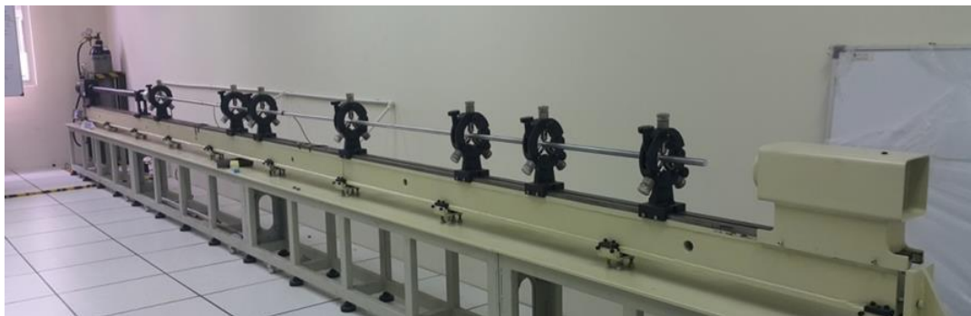
Fig. 1 - SHPB in UPNM's laboratory
