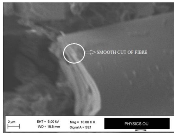
**Fig. 8 - SEM micrograph showing better surface quality (Smooth cut of fibre) of CFRP composite, when spindle speed is 4000rpm, feed rate is 200mm/min, and depth of cut is 0.5mm**
