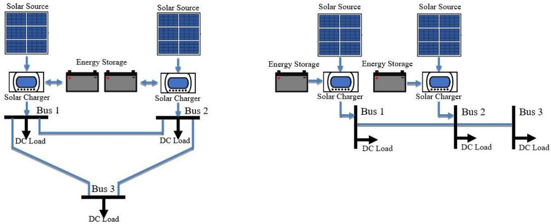
Fig. 1 - Model representation of (a) ring (b) radial DC micro-grid system
