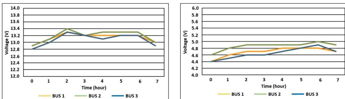
Fig. 4 - Distributed voltage each bus in the experimental of (a) ring and (b) radial DC microgrid system at 12 V<sub>DC</sub> level
