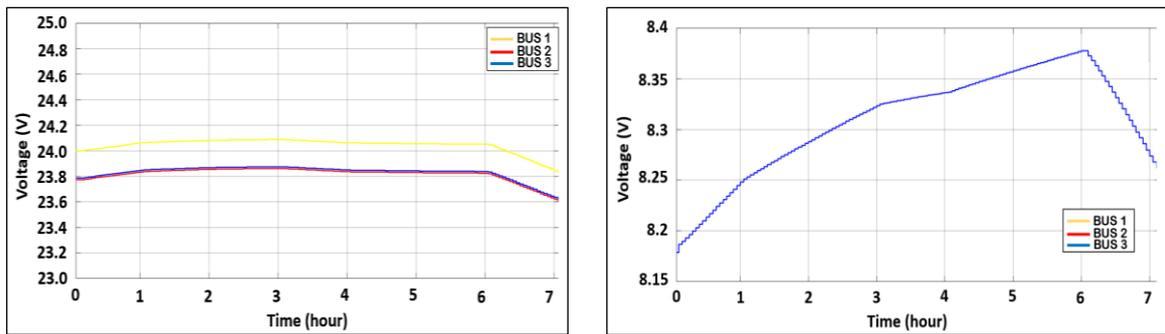
Fig. 5 - Distributed voltage each bus in the simulation of (a) ring and (b) radial DC microgrid system at 24 V<sub>DC</sub> level
