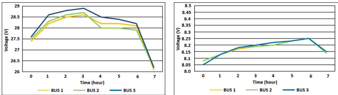
Fig. 6 - Distributed voltage each bus in the experimental of (a) ring and (b) radial DC microgrid system at 24 V<sub>DC</sub> level
