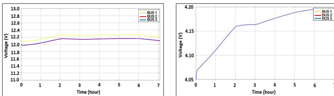
Fig. 3 - Distributed voltage each bus in the simulation of (a) ring and (b) radial DC micro-grid system at 12 V<sub>DC</sub> level
