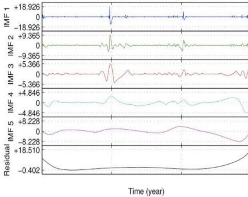
**Fig. 3 - Decomposed wind speed IMF1-IMF5**
