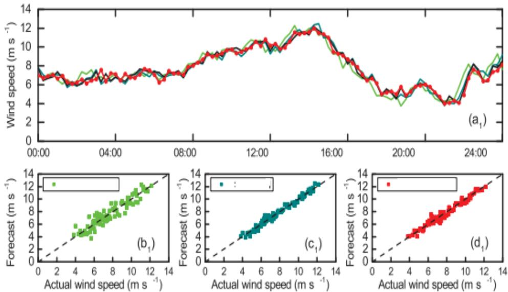
**Fig. 4 - Wind speed forecast results (a) IMF+GBM and ARIMA, b (Case 1) c (Case 2) and d Case (3)**
