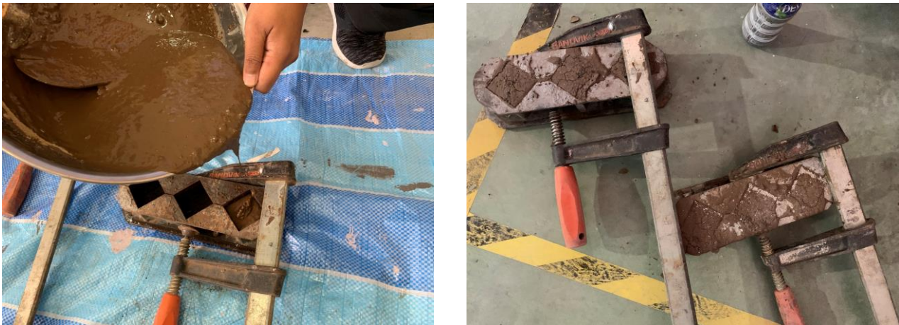
Fig. 7 - The geopolymer are labelled as Specimen 1-6 in the mould
