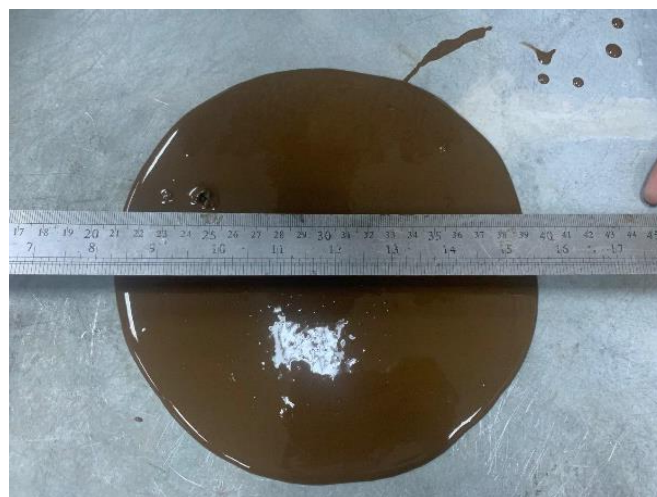
Fig. 3 - Measurement of d 1 and d 2 for geopolymer paste
