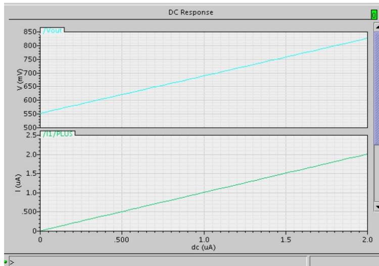
**Fig. 8 - DC response of three-stage inverter-based TIA**
