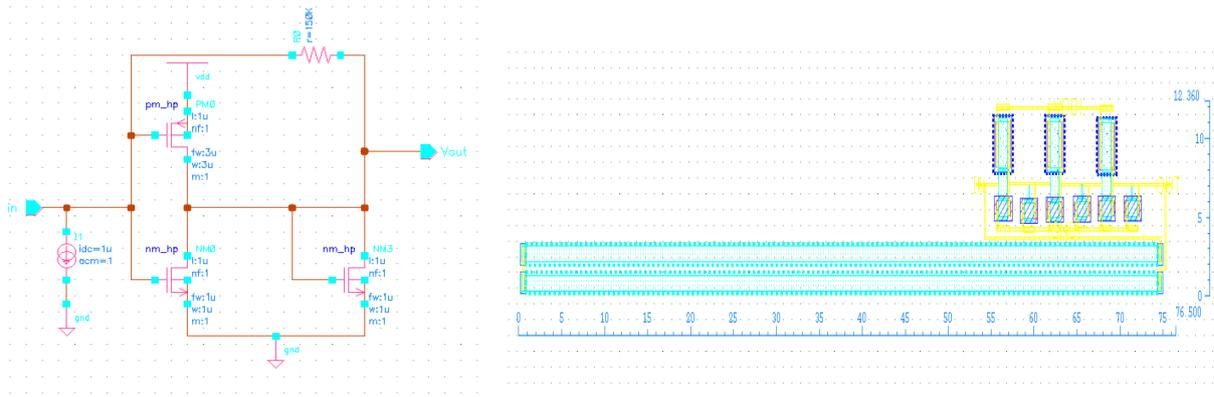
Fig. 6 - (a) Schematic for single-stage; (b) Layout of three-stage inverter-based transimpedance amplifier
