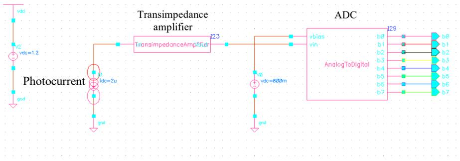
Fig. 10 - Full schematic diagram of monolithic light intensity sensor
