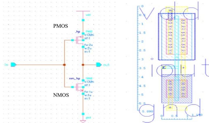
Fig. 5 - (a) Schematic diagram; (b) Layout of the inverter (1.170 μm x 5.890 μm)
