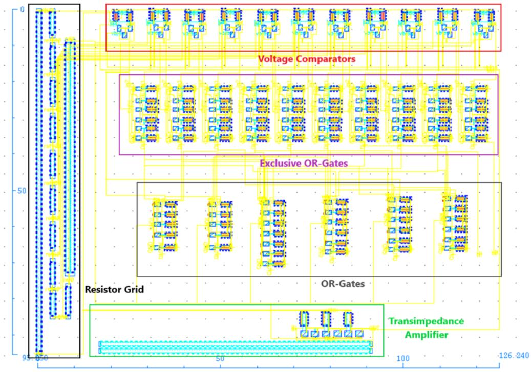
Fig. 11 - Full layout of monolithic light intensity sensor (126.240  $\mu\text{m}$  x 95.250  $\mu\text{m}$ )
