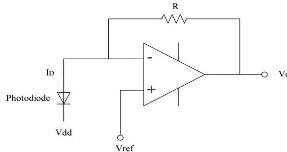
Fig. 4 - Diagram of a transimpedance amplifier
