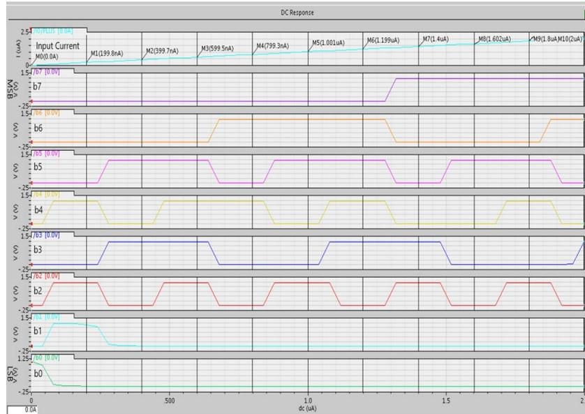
**Fig. 12 - Sample of binary output of the monolithic light intensity sensor**
