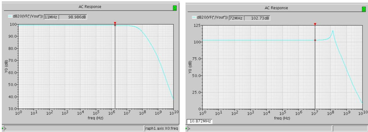
**Fig. 7 - (a) AC Response of single-stage inverter-based TIA; (b) AC Response of three-stage inverter-based transimpedance amplifier**
