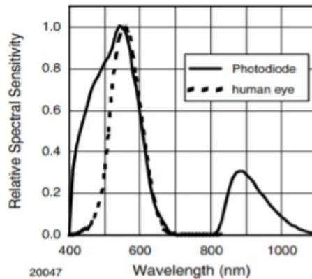
**Fig. 2 - Relative spectral sensitivity vs wavelength of the TEMD5510FX01 photodiode and the human eye [13]**
