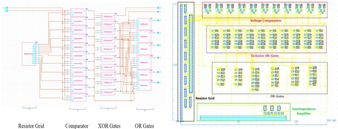
**Fig. 9 - (a) Schematic diagram of full ADC; (b) Layout of full ADC (127.350 μm x 94.580 μm)**
