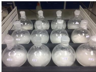
**Fig. 1 - Carbonation experiment carried out in a 250 mL round bottom flask placed on orbital shaker**
