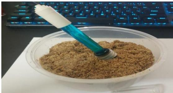
**Fig. 6 - Poking the end of pH Probe into the Soil Sample**
