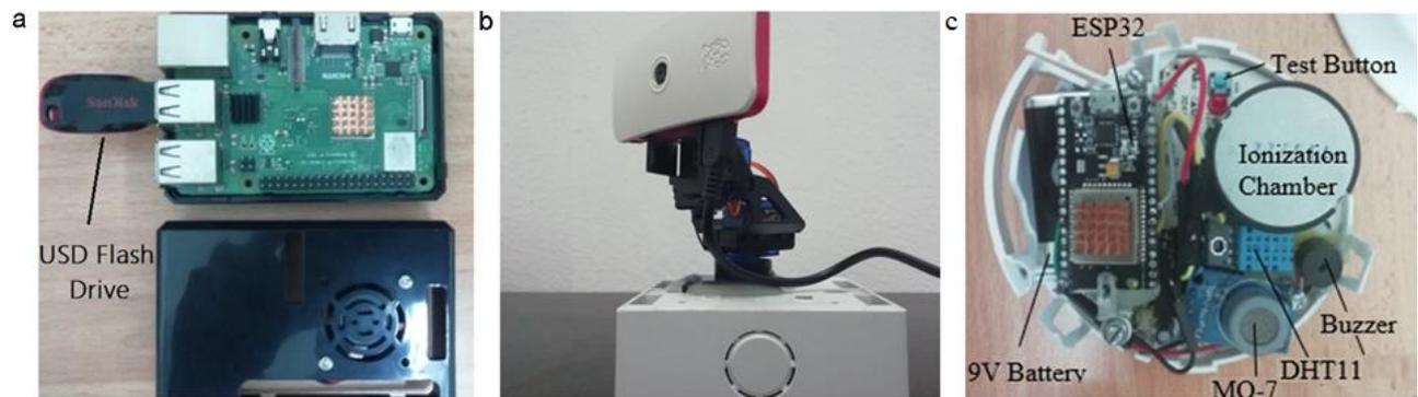
Fig. 6 - (a) Processing unit; (b) Surveillance unit; (c) Detector unit (inside view)
