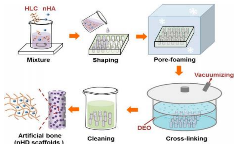
Fig. 10 - Schematic diagram of foam replication process in production of nano-hydroxyapatite (n-HA) with human-like collagen (HLC) scaffolds [116]
