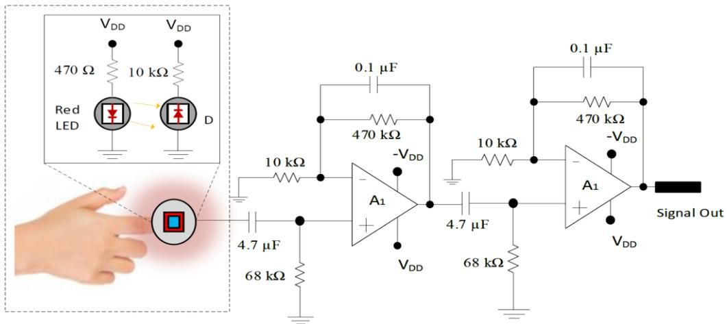
Fig. 3 - Bio signal conditioning circuit design
