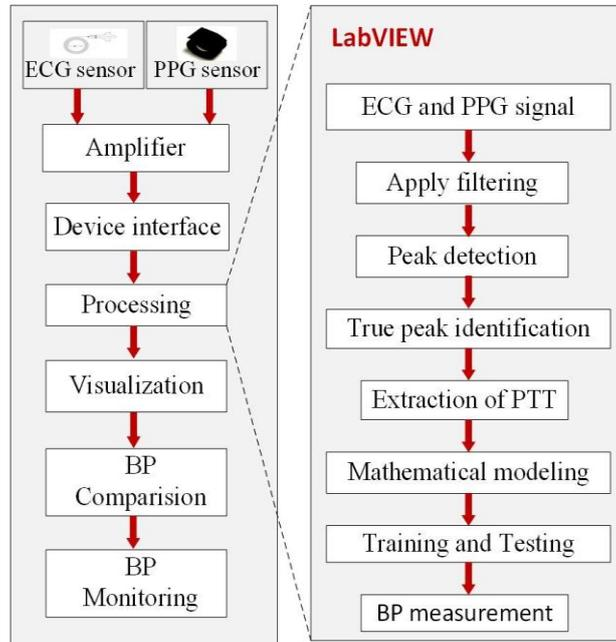
**Fig. 5 - Measurement system flow diagram depicting blood pressure measurement**
