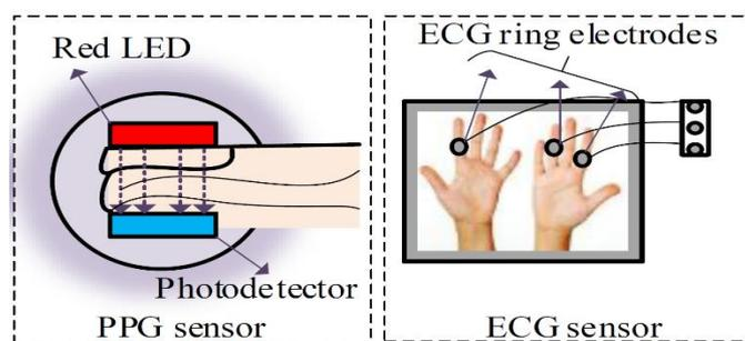
**Fig. 2 - PPG and ECG sensor configuration for signal acquisition**
