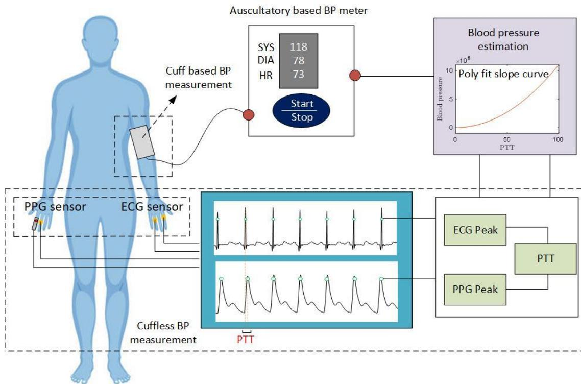
**Fig. 1 - Proposed system architecture for blood pressure measurement system**
