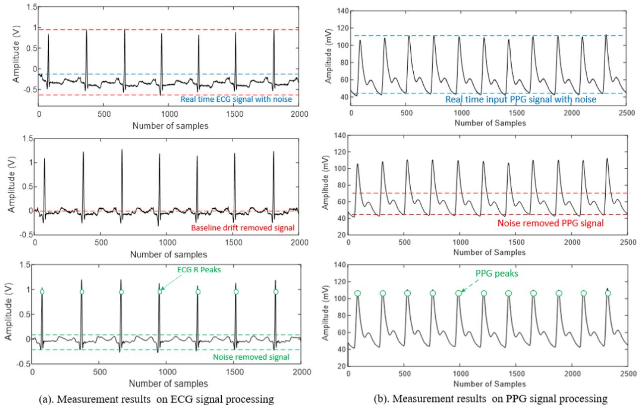
**Fig. 6 - Experiment results for ECG, PPG signal processing and feature extraction**
