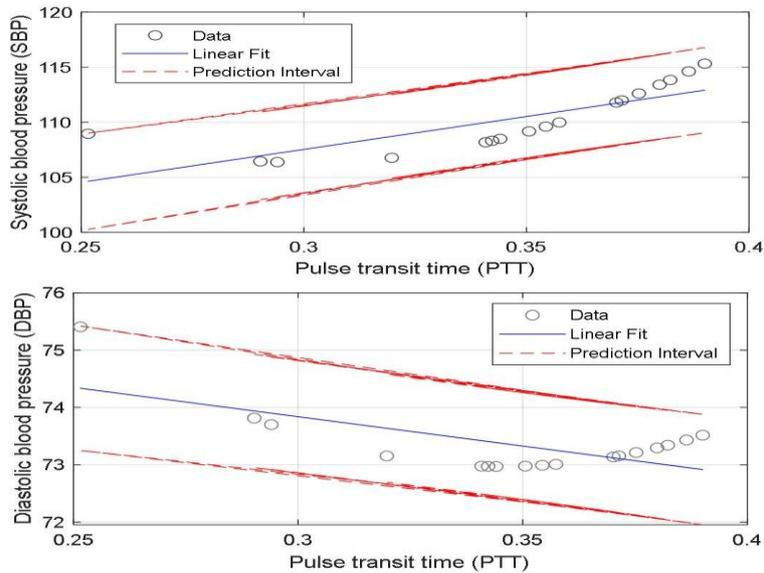
**Fig. 7 - PTT Vs Estimated blood pressure linear fit curve along with prediction interval. PTT is measured in terms of seconds**
