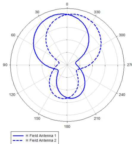
**Fig. 5 - H Fields for MIMO Antenna**
