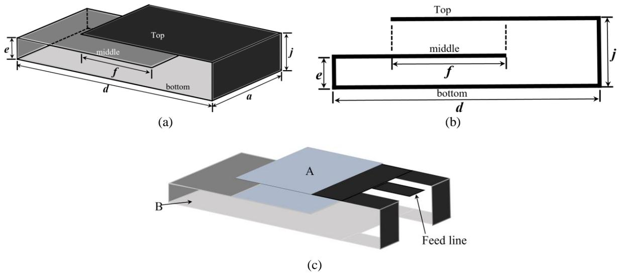
**Fig. 1 - Proposed Structure of the IMD antenna; (a) Dimension used to determine the resonant frequency of the antenna; (b) Side view of the antenna to create opposite G shape; (c) Illustration of the Isolated Magnetic Dipole Antenna**
