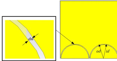
**Fig. 8 - Semi-circle slot structure etched on the ground layer**
