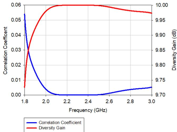
**Fig. 11 - Correlation Coefficient and Diversity Gain for MIMO antenna**
