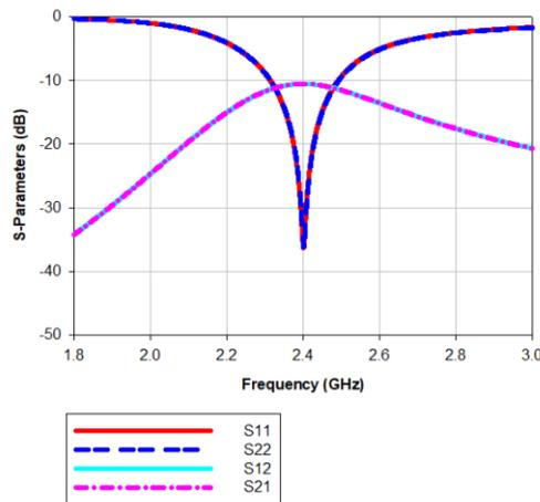
**Fig. 7 - S-Parameters without semi-circle slot on the ground layer**
