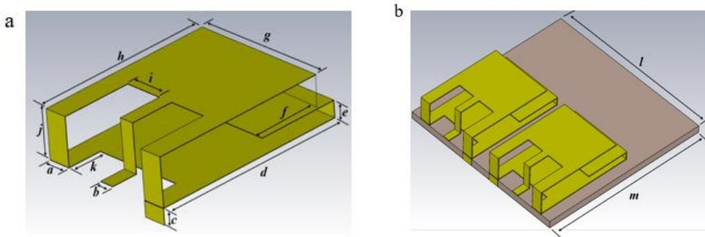
**Fig. 2 - Physical dimensions of patch antenna; (a) Antenna structure; (b) Antenna structure with the substrate layer**
