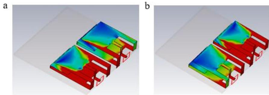
**Fig. 9 - Surface current of the antenna; (a) Antenna 1; (b) Antenna 2 without defective ground structure**
