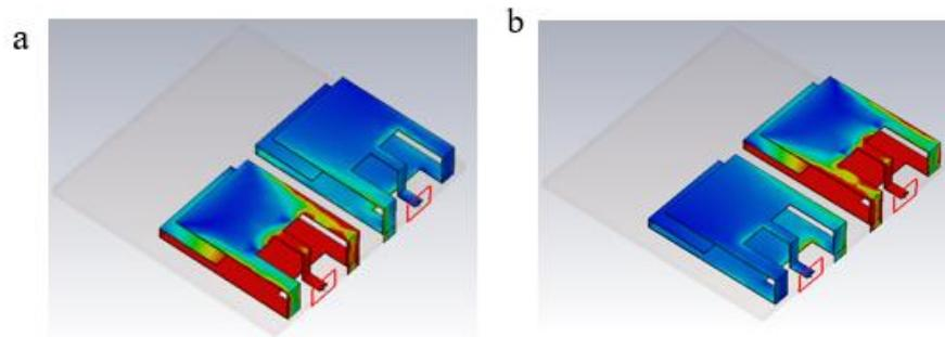
**Fig. 10 – Surface current of the antenna; (a) Antenna 1; (b) Antenna 2 with semi-circle slot**
