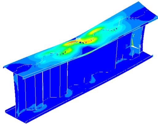
**Fig. 8 - Failure pattern of trapezoidal corrugated web**
