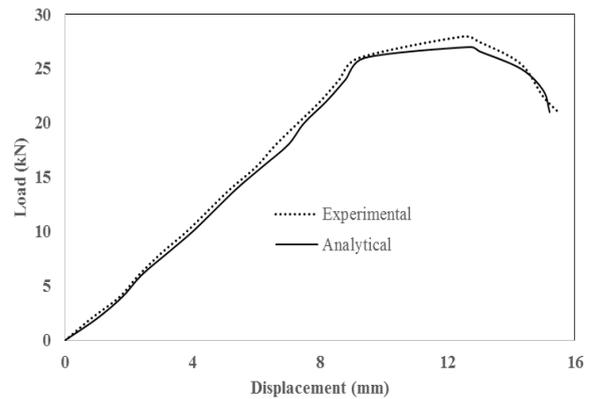
**Fig. 11 - Load vs deflection for trapezoidal corrugated web**
