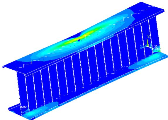
**Fig. 9 - Failure pattern of triangular corrugated web**
