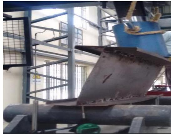
**Fig. 5 - Failure pattern of plain web**
