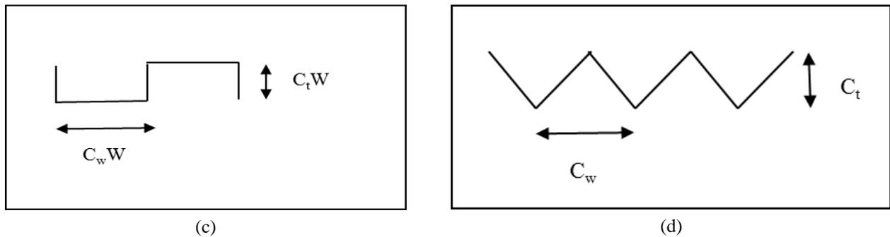
**Fig. 1 - Section Parameters (a) Plain Web; (b) Trapezoidal Corrugated Web; (c) Rectangular Corrugated Web; (d) Triangular Corrugated Web**
