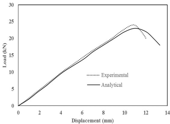
**Fig. 12 - Load vs deflection for rectangular corrugated web**
