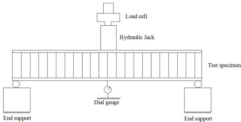
**Fig. 2 - Experimental setup of beam specimen**
