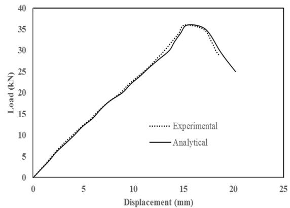
**Fig. 13 - Load vs deflection for triangular corrugated web**
