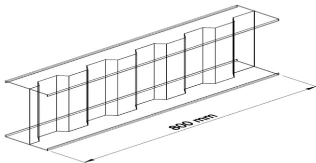
**Fig. 3 - Diagrammatic representation of trapezoidal corrugated web lipped I beam**
