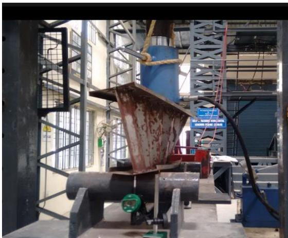
**Fig. 4 - Failure pattern of trapezoidal corrugated web**
