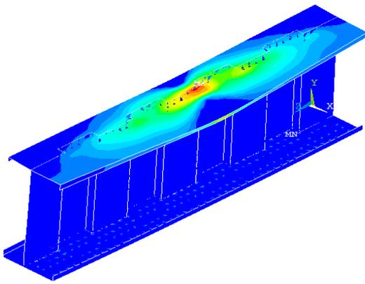
**Fig. 7 - Failure pattern of plain web**
