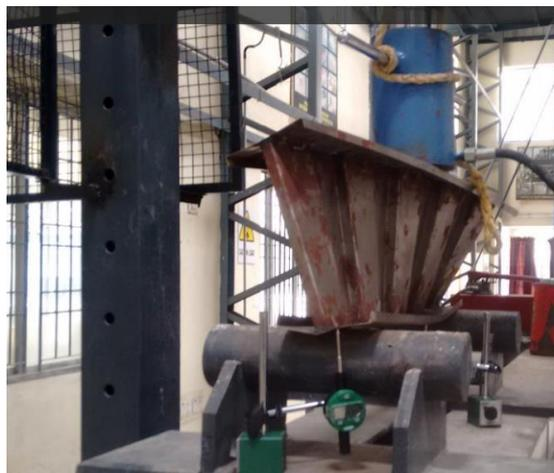
**Fig. 6 - Failure pattern of rectangular corrugated web**
