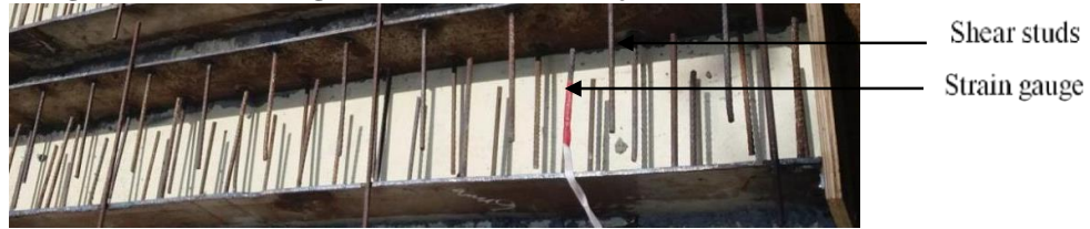
Fig. 3 - SCS beam with normal shear studs
