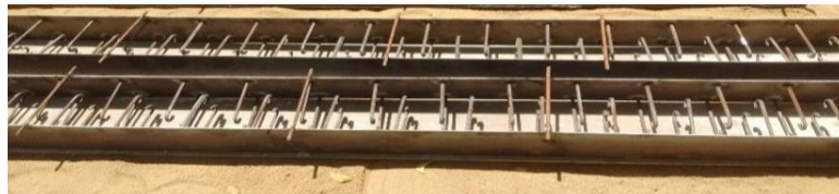
Fig. 4 - SCS beam with j-hooks shear studs
