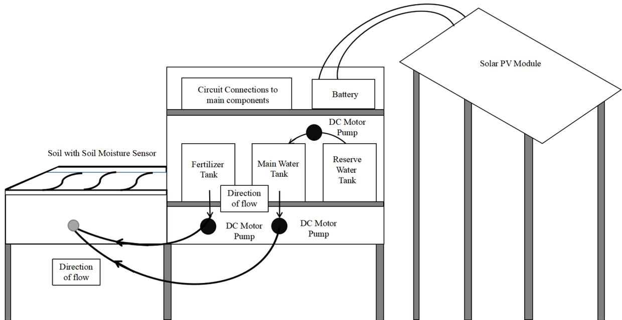
**Fig. 2 - The solar powered automated irrigation and fertigation system**
