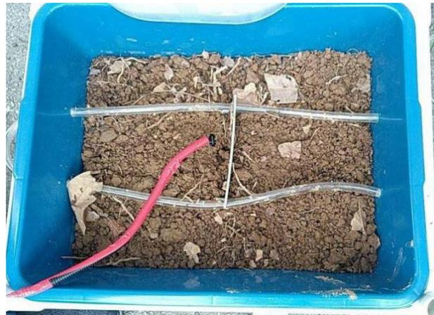
**Fig. 7 - Top view of soil area with drip system and moisture sensor**
