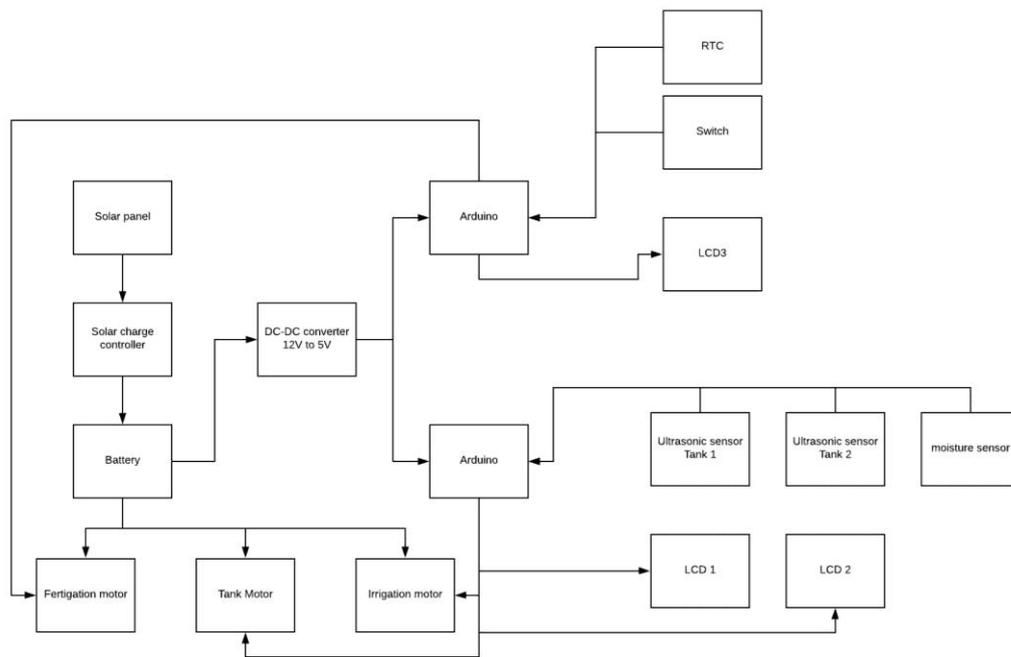
**Fig. 3 - The solar powered automated irrigation and fertigation system**
