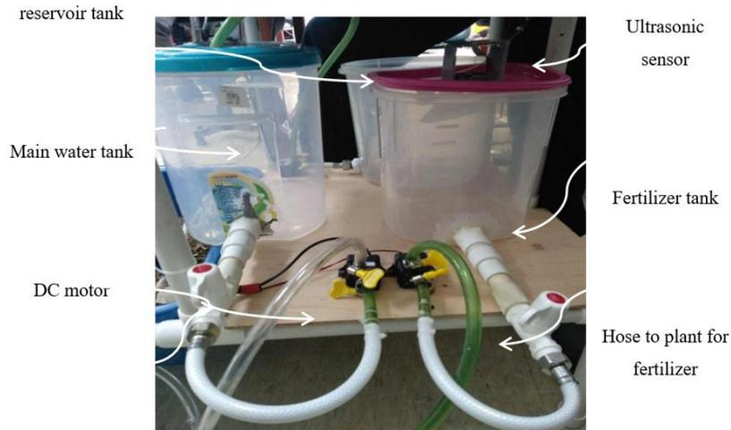
**Fig. 6 - The automated solar powered irrigation and fertigation system**
