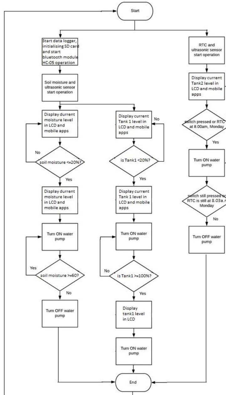
**Fig. 4 - The solar powered automated irrigation and fertigation system**
