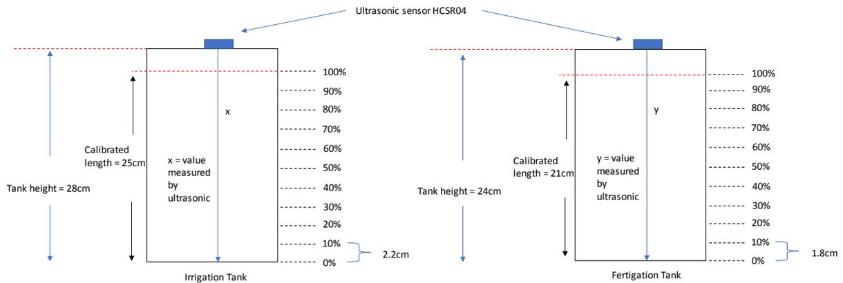
**Fig. 5 - Ultrasonic sensors calibration**
