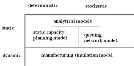
Fig. 1 Different modeling tools to model manufacturing system
