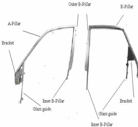
Fig.7 Front door-sash for car
