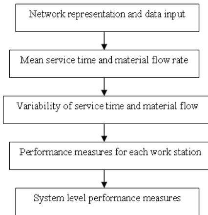
Fig. 2 Procedure to calculate performance measures on spreadsheet model
