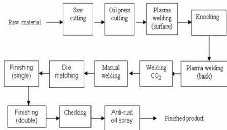
Fig.6 A schematic of workstations in an assembling production line
