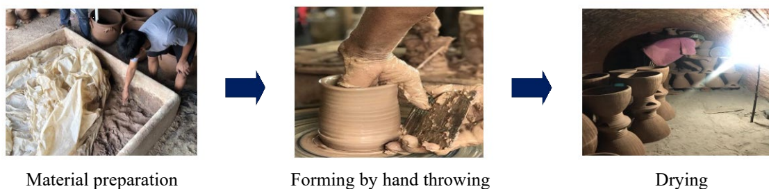
Fig. 2 - A general pottery forming process
