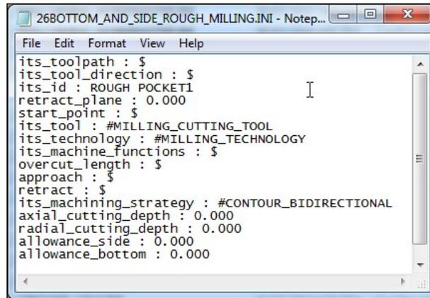
Fig. 6 - Configuration for bottom and side rough milling
