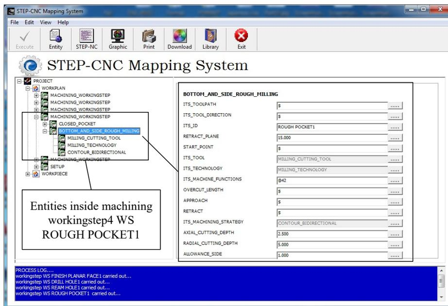
Fig. 7 - Interface for bottom and side rough milling
