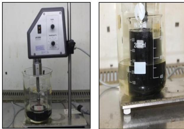
Fig. 2 - Pre-dispersion process using Hielscher Ultrasonic Homogenisers UP200s
