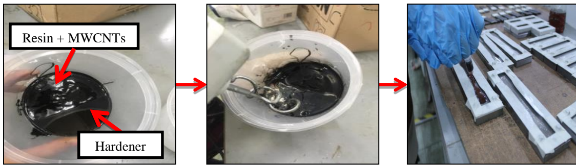
Fig. 4 - Preparation of modified epoxy grout
