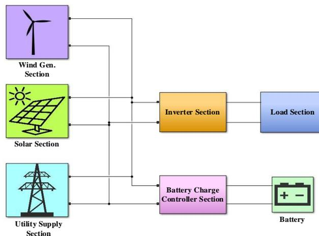
**Fig. 4 - Simulink/ MATLAB model of the hybrid system**
