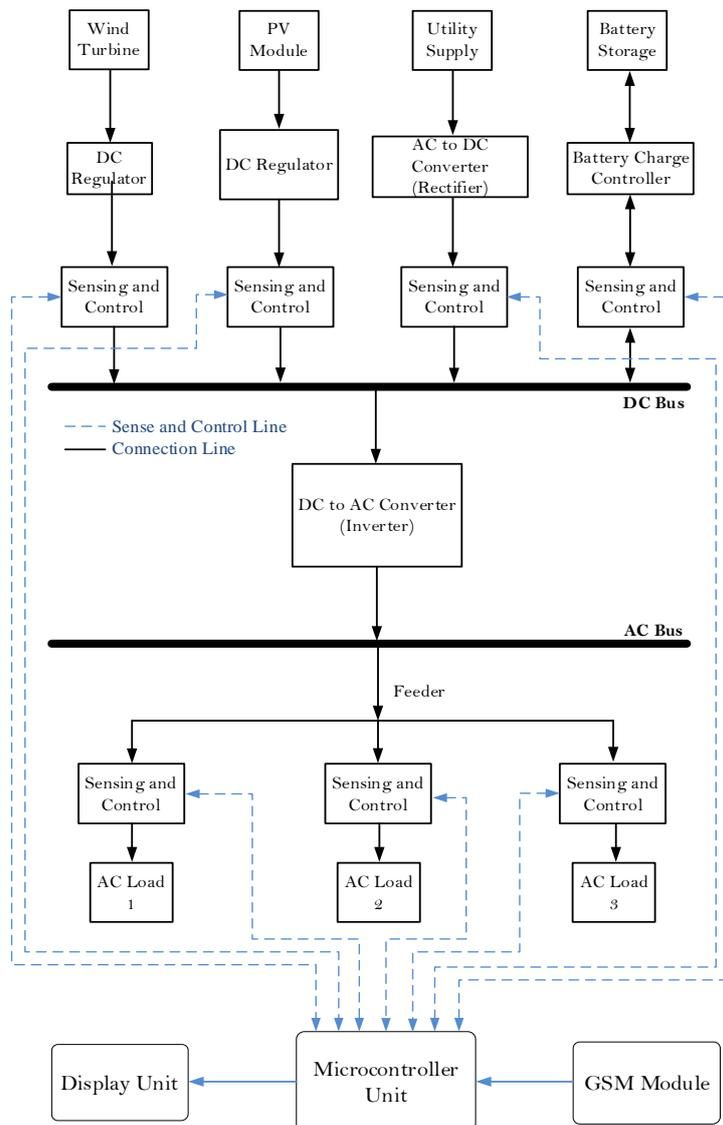
Fig. 3 - The complete model of the system
