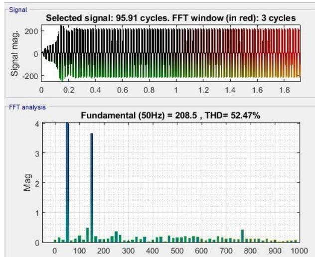
Fig. 10 - THD of the output voltage from the SPWM inverter
