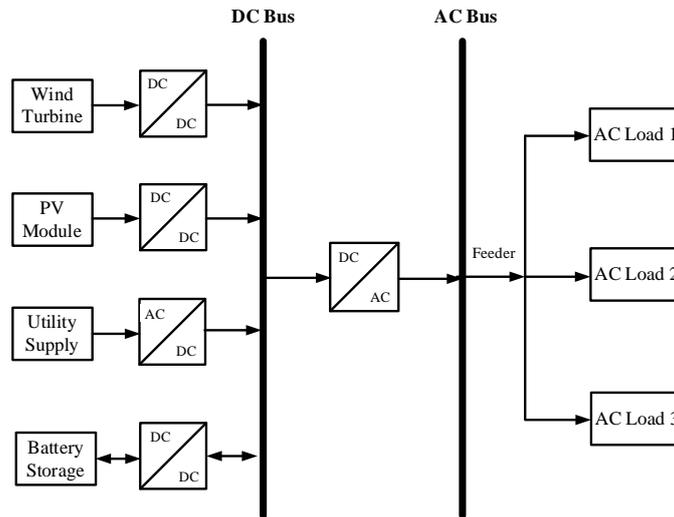
Fig. 1 – structure of proposed hybrid system
