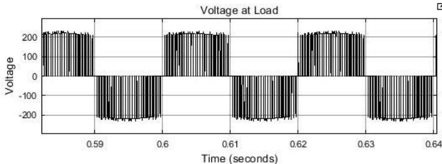
Fig. 7 - Output voltage from the SPWM inverter (close-up view)
