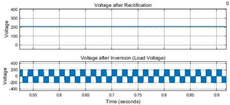
Fig. 11 - Voltage after rectification of WAPDA supply, and load voltage
