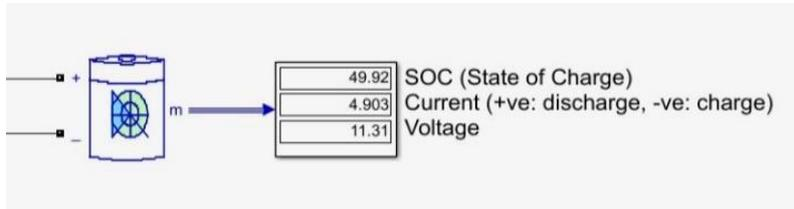
**Fig. 13 - Battery in its discharging state**
