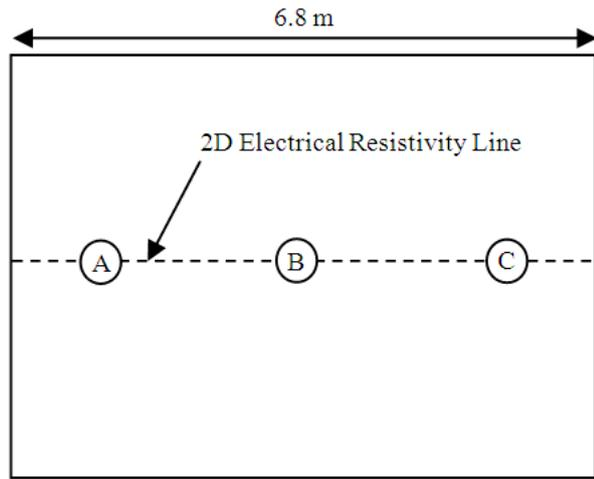
Fig. 2 Schematic diagram (Plan view) of the position of soil sampling and resistivity line alignment.
