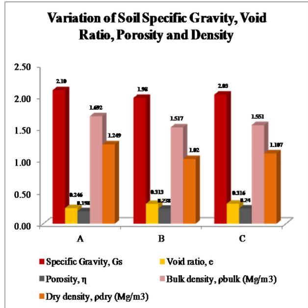
Fig. 5 Variations of BGP with particular reference to specific gravity, void ratio and porosity.
