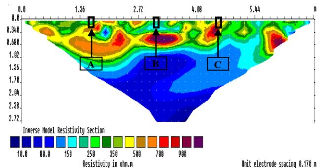
Fig. 3 2D electrical resistivity section and localized extracted ERV (A, B and C) used for further detail study.
