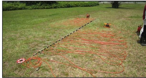
Fig. 1 2D resistivity data acquisition in progress.
