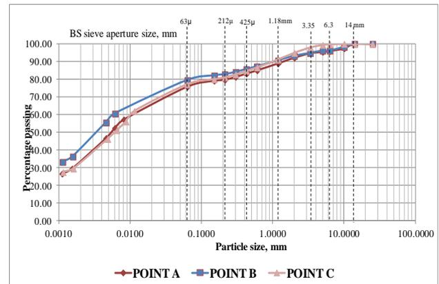
Fig. 4 PSD curve for soil sample at point A, B and C.
