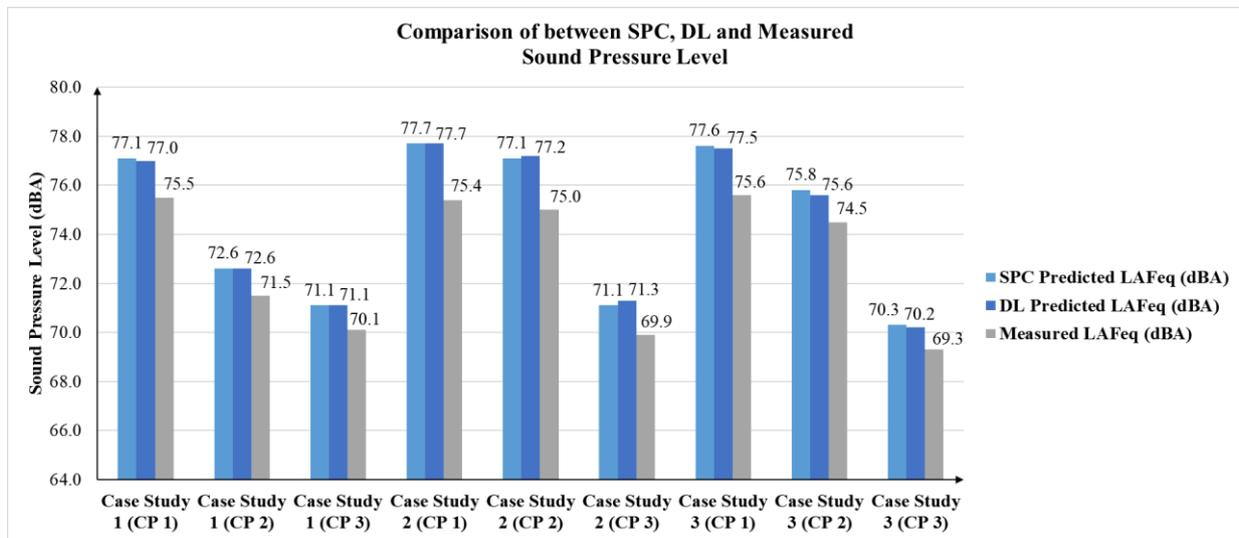
**Fig. 5 - Comparison between prediction and measure sound pressure level**
