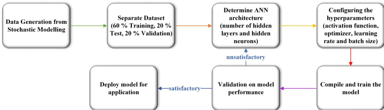
Fig. 2 - Framework of Artificial Neural Network
