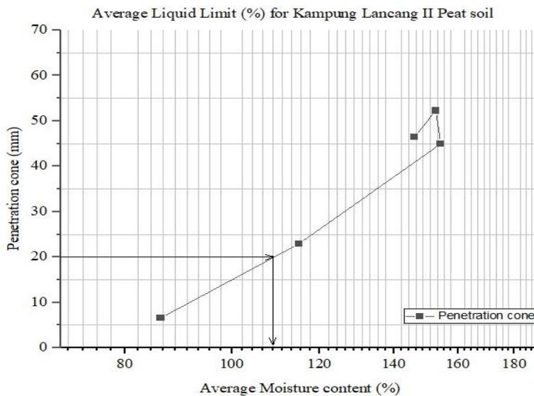
Fig. 9 - The liquid limit for Kampung Lancang II peat soil
