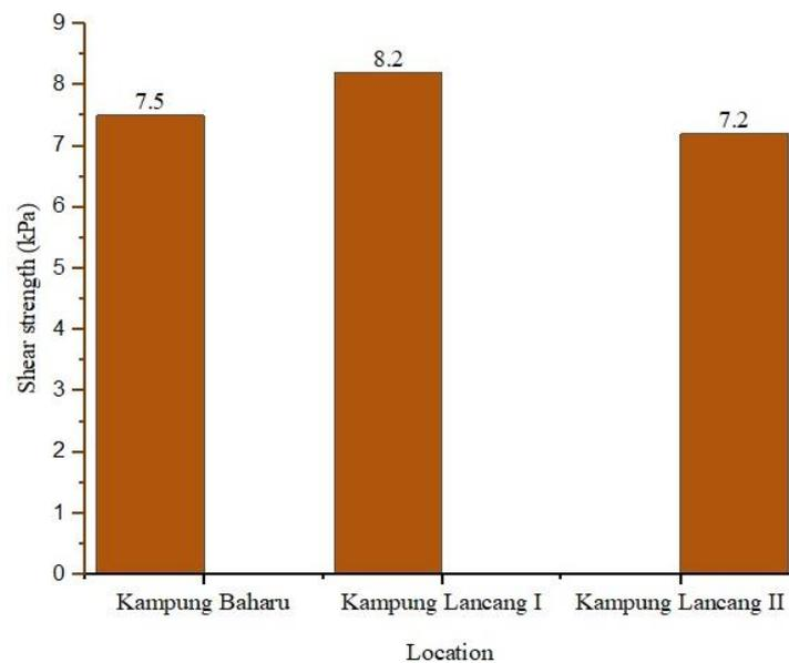
Fig. 5 - The shear strength (kPa) for peat soil
