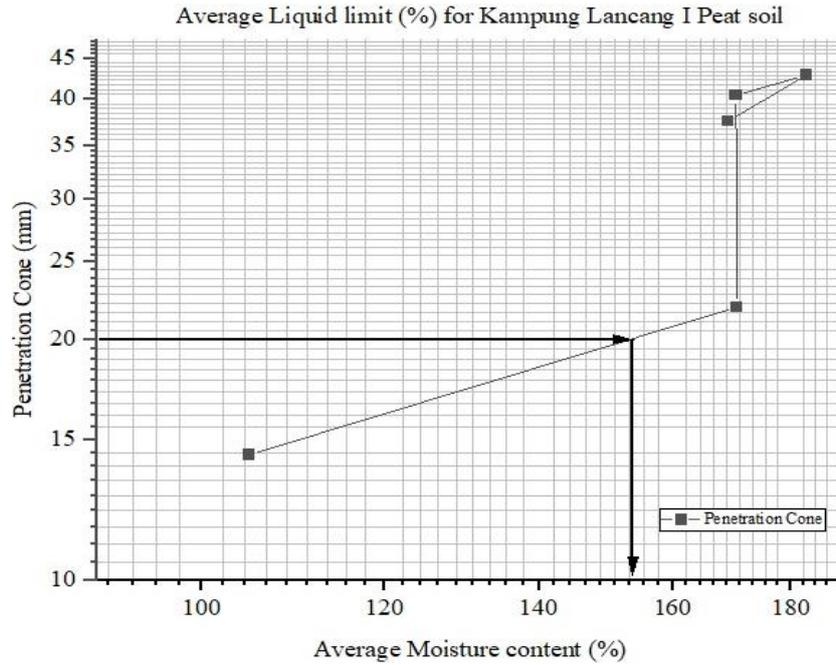
Fig. 8 - The liquid limit for Kampung Lancang I peat soil
