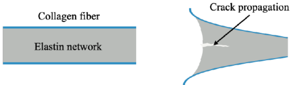
Fig. 5 - The elastin network between the collagen fibers break during tissue tearing
