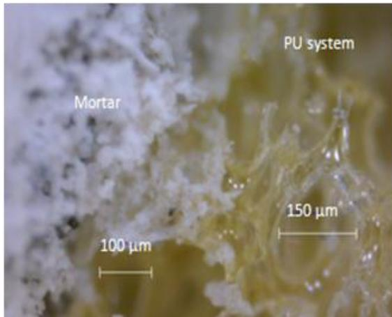
Fig. 6 Interfacial zones between concrete and PU observed using optical microscope at 500× magnifications.
