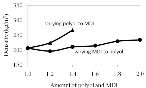
Fig. 1 The effects of varying PKO-p and MDI on the density of rigid PU
