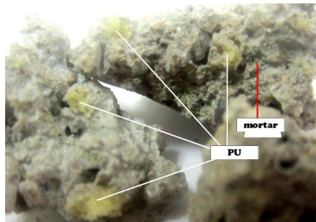
Fig. 5 Polyurethane (PU) covered by cement paste in the broken fragment of concrete.
