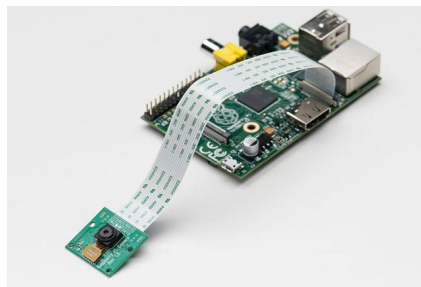
Fig. 4 - Connection of Raspberry-pi 3B and camera module V2
