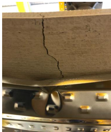
Fig. 12 - Cracking occur at mid-span
