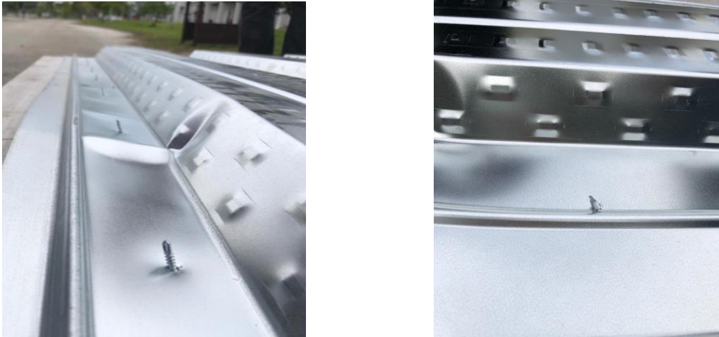
Fig. 13 - Shearing of screw connector
