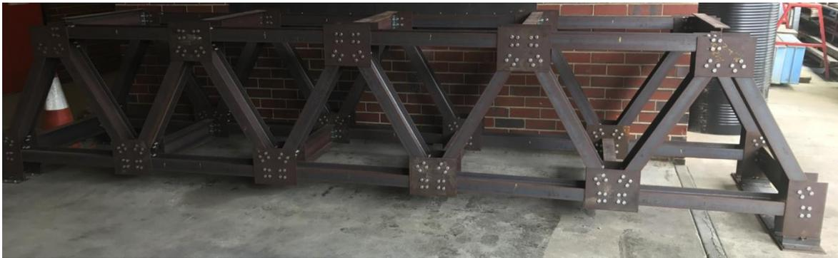
Fig. 2 - Laboratory scaled steel truss bridge structure
