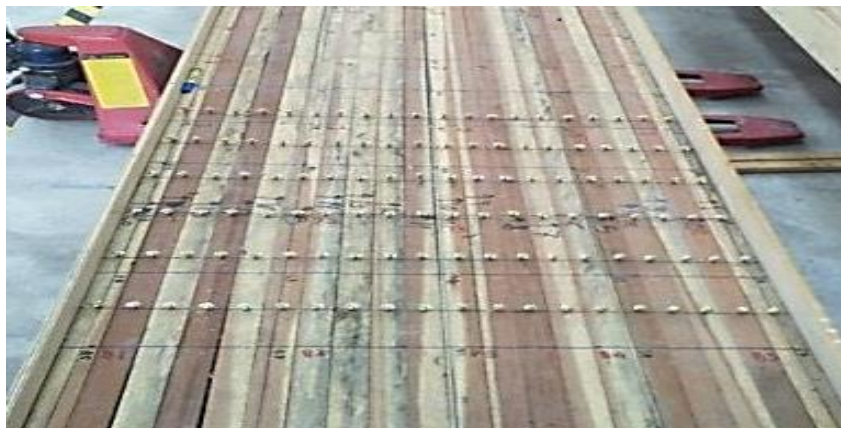
Fig. 3 - Screws as the connector
