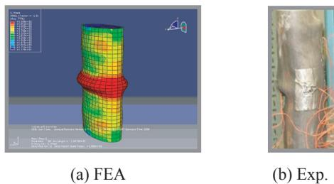
Fig. 3 Deformation shape from FEA and experimental
