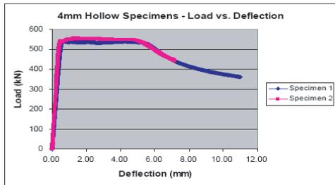
Fig. 2(b): Experimental results for 4 mm specimen thickness [12]
