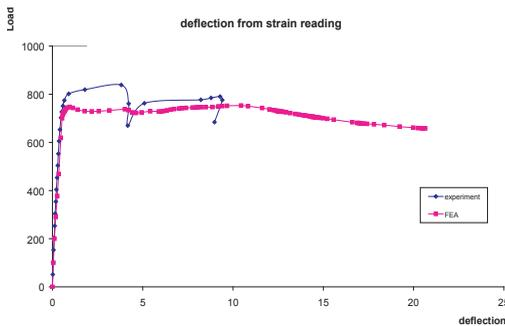
Fig. 4 Load-deflection curve for elliptical CFT column with 4mm thickness.
