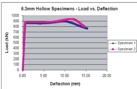
Fig. 2(d): FE results for 6.3 mm specimen thickness [12]
