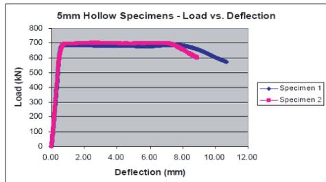
Fig. 2(c): FE results for 5 mm specimen thickness [12]
