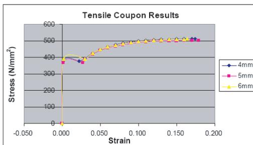
Fig.1 Stress-strain curve from coupon test
