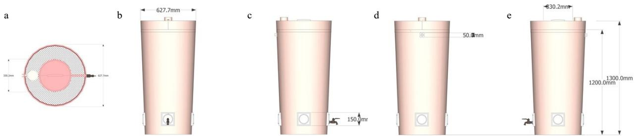
Fig. 4 - a) Plan; b) front elevation; c) right elevation; d) rear elevation; e) left elevation
