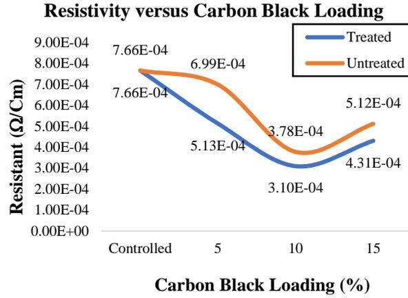
Fig. 4 - Resistivity of various carbon black loading filled silicone
