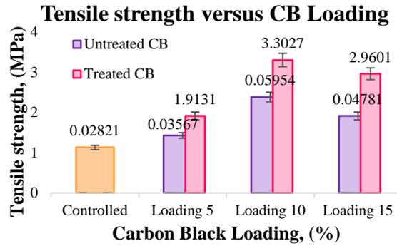
Fig. 2 - Tensile strength with various loading of CB
