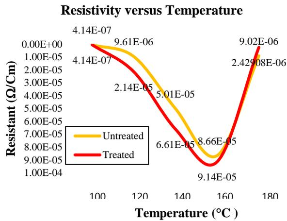
Fig. 6 - Resistivity of temperature for various loadings of carbon black filled silicone at elevated temperature
