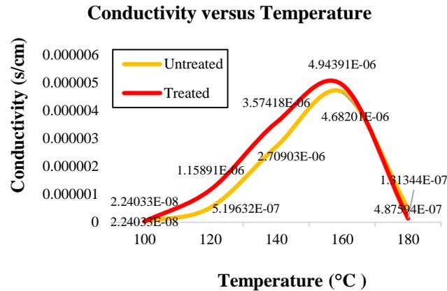
**Fig. 7 - Conductivity versus temperature for untreated carbon black and treated carbon black filled silicone**
