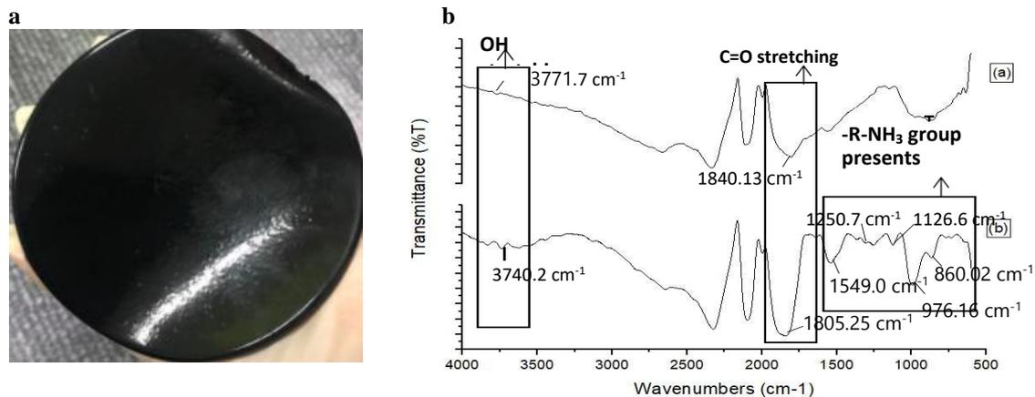
Fig. 1 – (a) Sample of silicone electrical conductive adhesives filled carbon black; (b) FTIR spectra of treated and untreated carbon black; (c) untreated CB; (d) treated CB
