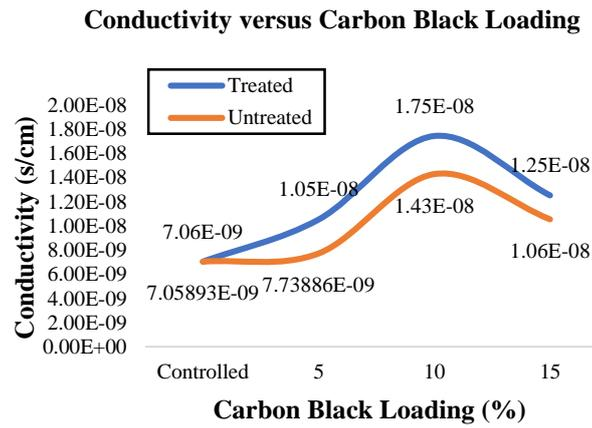
Fig. 5 - Conductivity of various loadings of untreated and treated carbon black filled silicone
