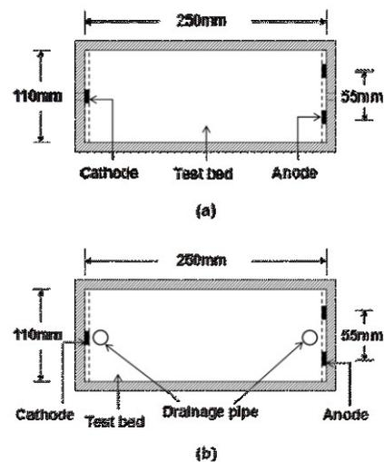
Fig. 7 Plan of test tank showing the 2anodes-1cathode configuration: (a) Drainage at bottom of test bed (b) Drainage through drainage pipe [10].
