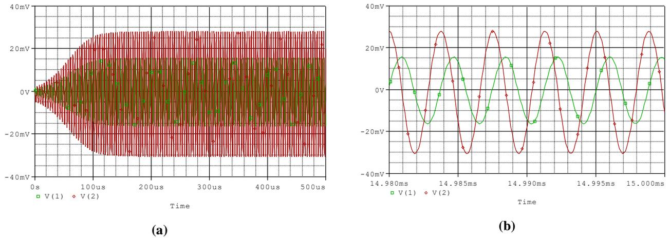
Fig. 3 - (a) Transient waveform and (b) steady-state response of oscillator circuit in Fig. 2
