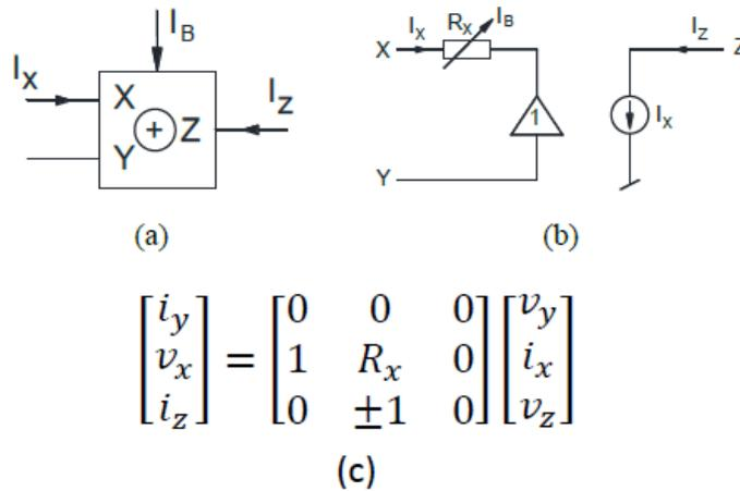
**Fig. 1 - CCCII (a) Symbolic notation (b) corresponding circuit and (c) port characteristic matrix of CCCII**
