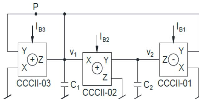
**Fig. 2 - Proposed electronically tunable sinusoidal quadrature oscillator circuit**
