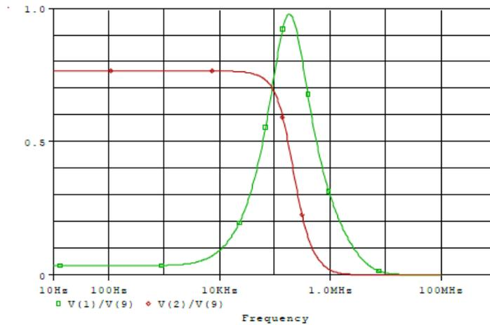
**Fig. 5 - Frequency response of the low-pass and band-pass filter realized from the circuit in Fig. 2 after modification**
