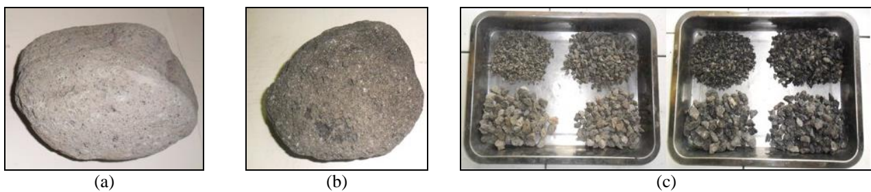
Fig. 1 - (a) Pumice; (b) scoria, and; (c) the gradation of pumice and scoria coarse aggregates
