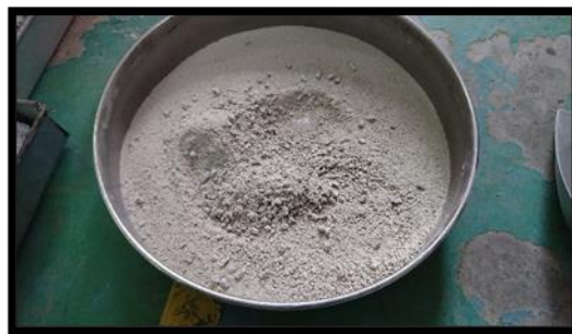
Fig. 1 - RFA sieved passing 5 mm sieve
