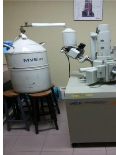
Fig. 4 - Scanning Electron Microscope (SEM) machine - JOEL JSM-630LV
