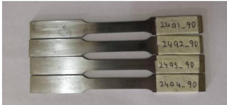
Fig. - 1 Example of tensile specimens
