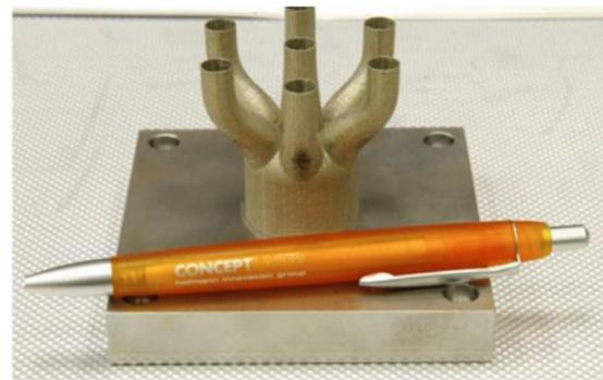
**Fig. 64 - Metal rocket injector part for their next-generation Space Launch System (SLS) J-2X engine [49]**
