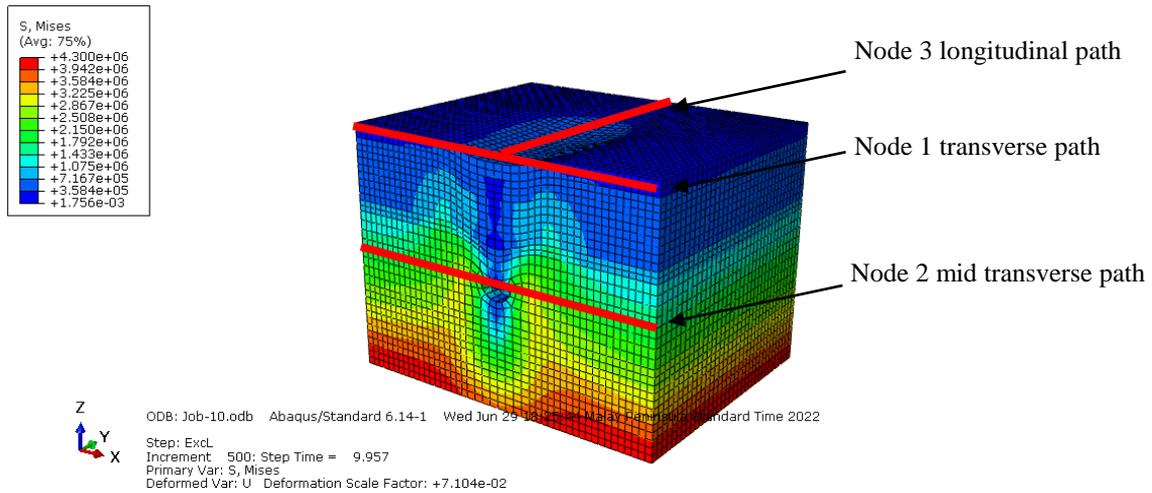
**Fig. 2 - Stress reaction due to mining and path of the node series taken to retrieve the results**
