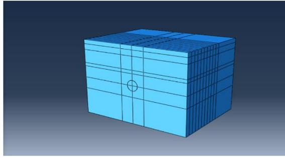
Fig. 2 - 3D model of the soil tunnel with the proposed tunnel diameter in ABAQUS software
