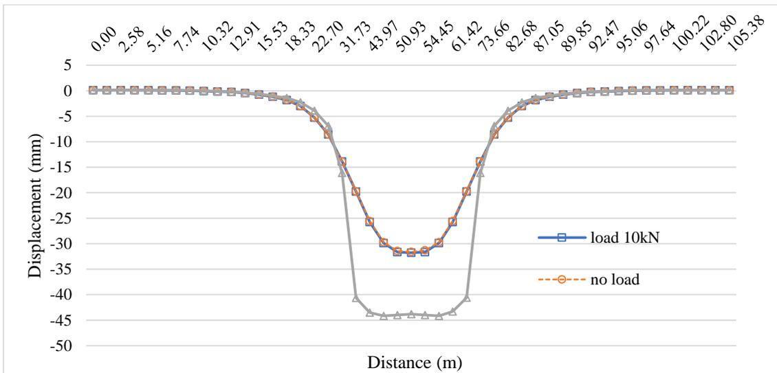
**Fig. 6 - Ground settlement in the transverse axis direction**
