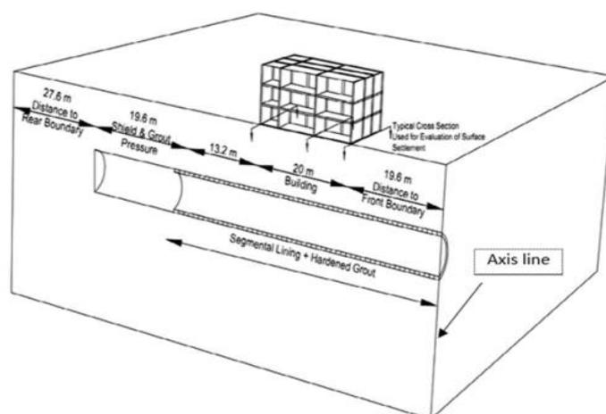
**Fig. 1 - Building and tunnel [7]**
