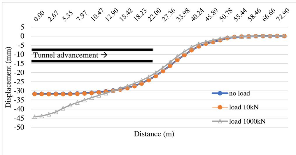
**Fig. 7 - Ground settlement in the transverse axis direction**
