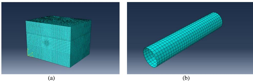
Fig. 1 - Meshing of : (a) soil block model and (b) tunnel model
