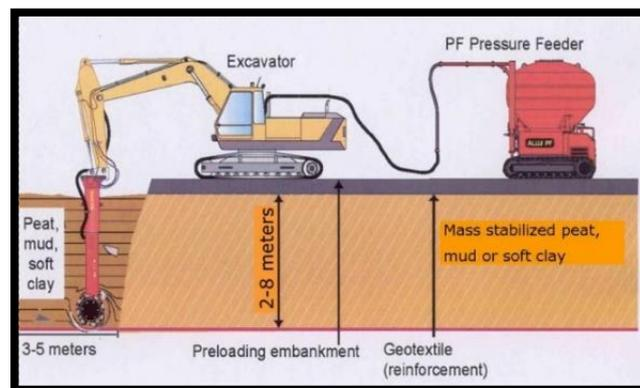
Fig. 3 - Mass stabilization method in peat soil
