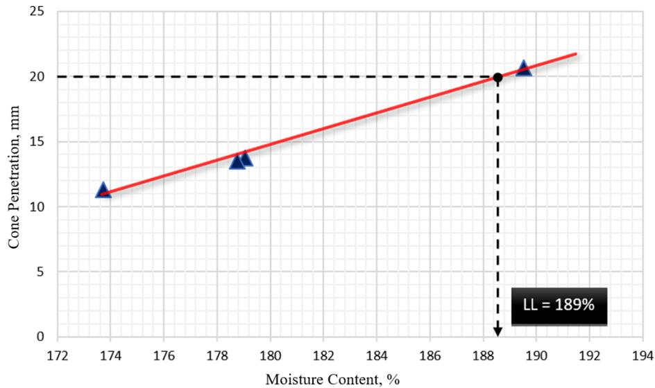
**Fig. 6 - Graph cone penetration against moisture content**
