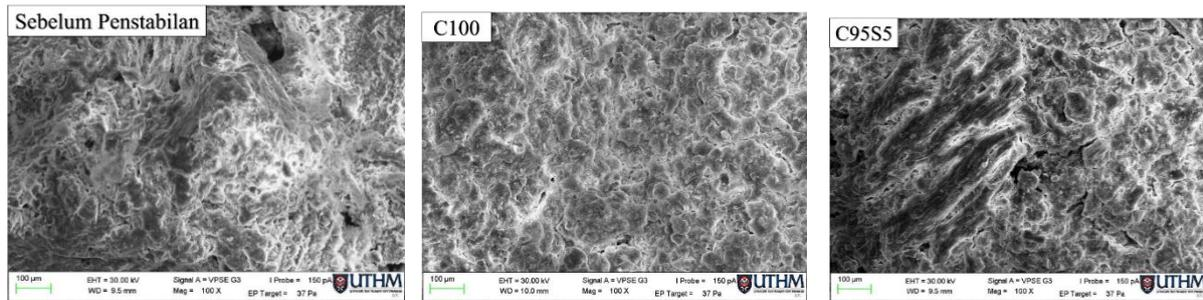
**Fig. 9 - SEM images for samples before and after stabilization**
