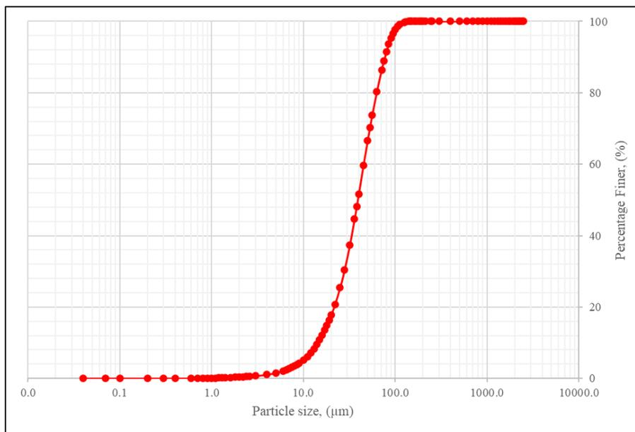
**Fig. 8 - Particle size distribution graph for SCBA material**
