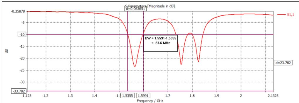
**Fig. 5 - The Simulated result of bandwidth FR-4 substrate**
