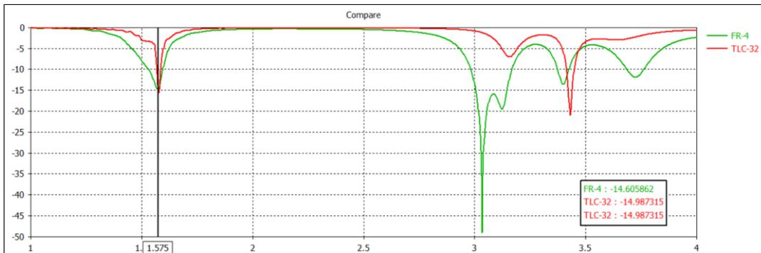
Fig. 9 - The simulated result of reflection coefficient of FR-4 and Taconic TLC-32 for truncated microstrip patch antenna with an Inset Feed
