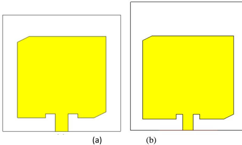
**Fig. 3 - The proposed antenna with inset feed design using 2 different substrate material (a) FR-4; (b) Taconic TLC-32**
