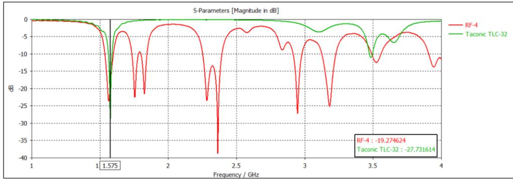
**Fig. 4 - Simulated result of return loss ( $S_{11}$ ) FR-4 and Taconic TLC-32 substrate**
