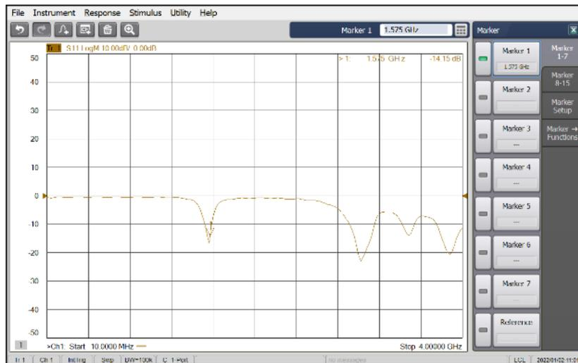
**Fig. 15 - Measurement result of return loss ( $S_{11}$ ) and bandwidth FR-4 substrate**
