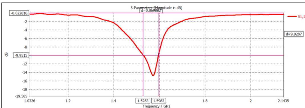
Fig. 10 - Simulated result of bandwidth of FR-4 for truncated microstrip patch antenna with an Inset Feed
