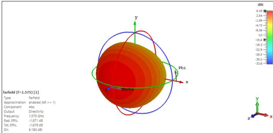
Fig. 8 - Simulated result of gain for Taconic TLC-32
