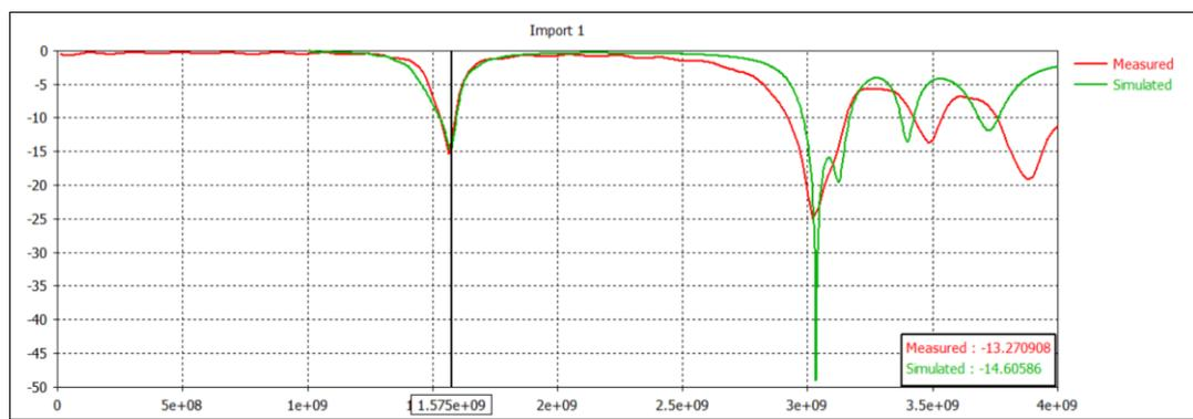
**Fig. 16 - Comparison of simulated and measured result for FR-4 substrate**
