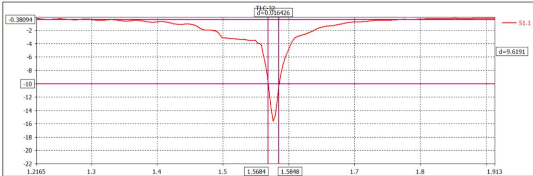
**Fig. 11 - Simulated result of bandwidth of Taconic TLC-32 for truncated microstrip patch antenna with an Inset Feed**
