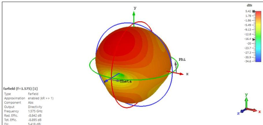
**Fig. 7 - Simulated result of gain for Taconic TLC-32**
