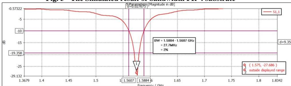
**Fig. 6 - Simulated result of bandwidth for Taconic TLC-32**
