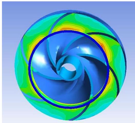
**Fig. 3 - Distribution of Pressure at Impeller Inlet**
