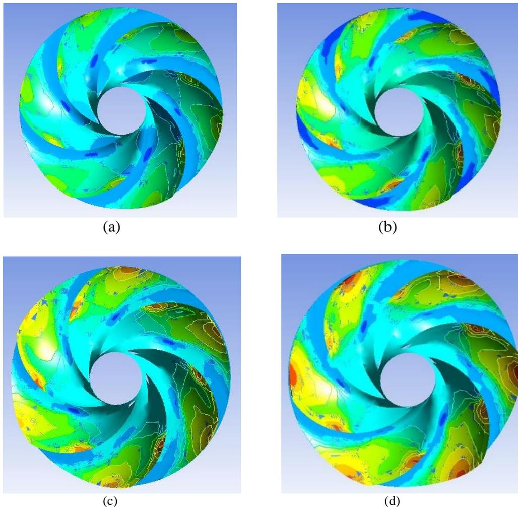
**Fig. 4 - Distribution of Cavity Volume Fraction in Impeller. (a)  $H_{NPSHa} = 2.09\text{ m}$ , (b)  $H_{NPSHa} = 1.43\text{ m}$ , (c)  $H_{NPSHa} = 1.32\text{ m}$ , (d)  $H_{NPSHa} = 1.21\text{ m}$**
