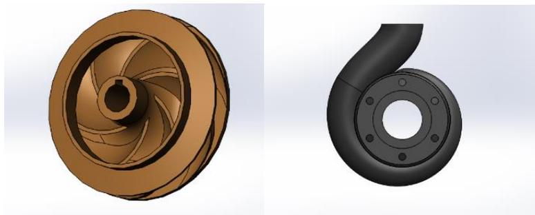
**Fig.1 - 3D modelling of Closed Impeller and Casing**
