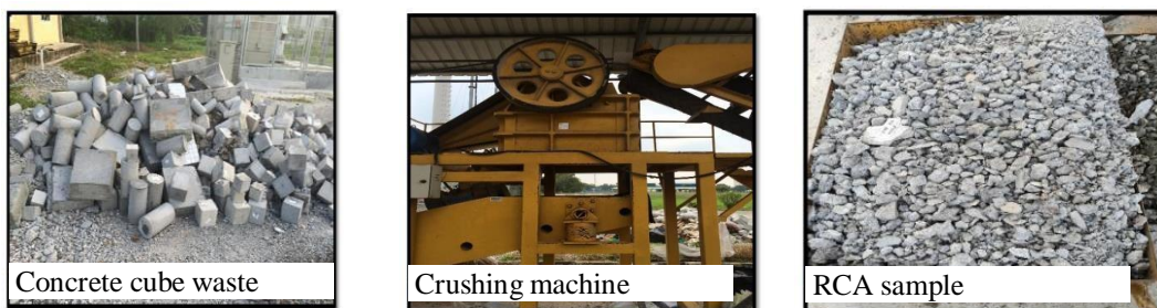
Fig. 1 - The process for crushing concrete cube into recycled concrete aggregate
