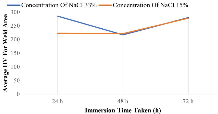
Fig. 6 - Graph average HV against immersion time taken for weld area
