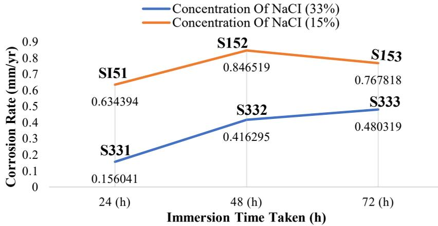
Fig. 5 - Graph corrosion rate against immersion time taken
