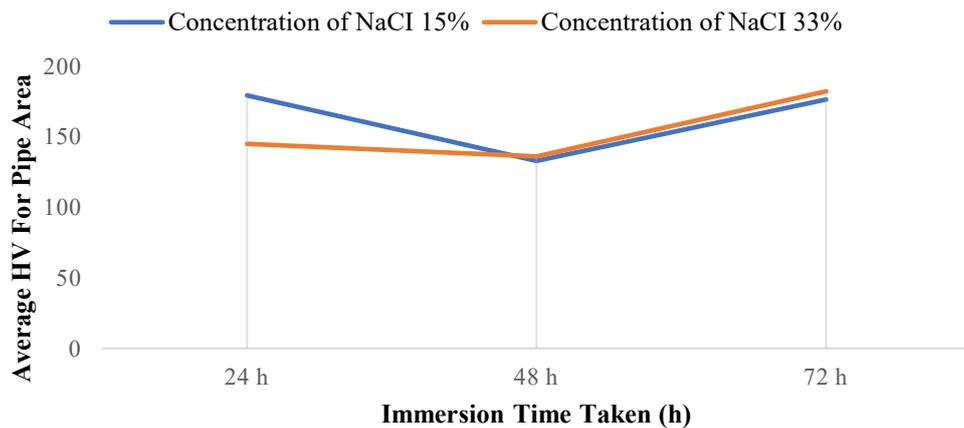
Fig. 7 - Graph average HV against immersion time taken for pipe area
