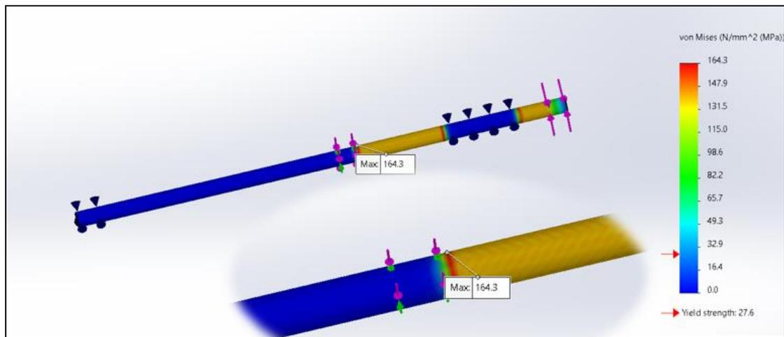
**Fig. 4 - Stress distribution of aluminium threaded shaft (8 Nm)**
