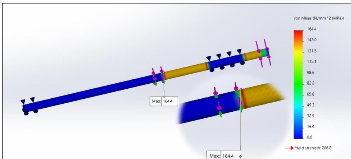
**Fig. 5 - Stainless steel threaded shaft's stress distribution (8 Nm)**
