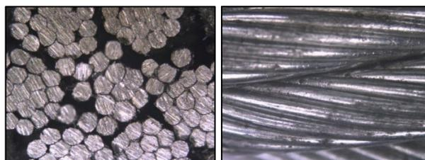
**Fig. 7 - Condition of cable wire protected using rubber hose and lubrication at x15 magnification**
