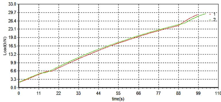
**Fig. 2 - Load vs time result for guy wire A1 and B1**
