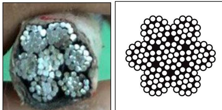
Fig. 1 - Construction of guy wire samples
