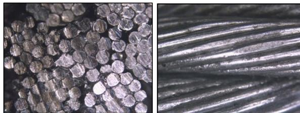
**Fig. 5 - Condition of cable wire at x15 magnification protected with lubrication**
