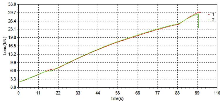
**Fig. 3 - Load vs Time result for guy wire A2 and B2**
