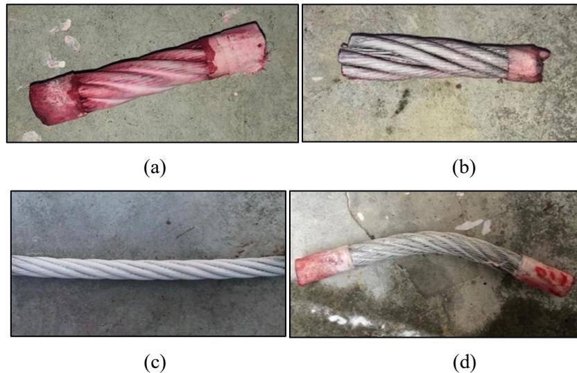
**Fig. 8 - Result of dye penetrant testing**
