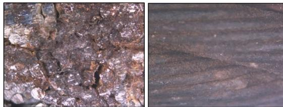
**Fig. 4 - Rust formation of cable wire at x15 magnification without protection**
