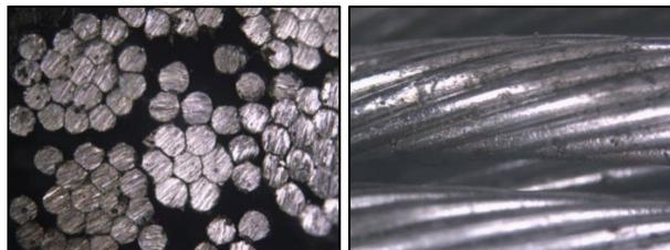
**Fig. 6 - Condition of cable wire rubber hose protected at x15 magnification**
